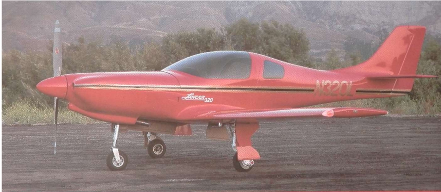
Lancair 320, 2 Plätze, 160 PS, Cruise 390 km/h, Range 2'330 km, 8 l/100 km «Until Ferrari builds an airplane, this is it»
